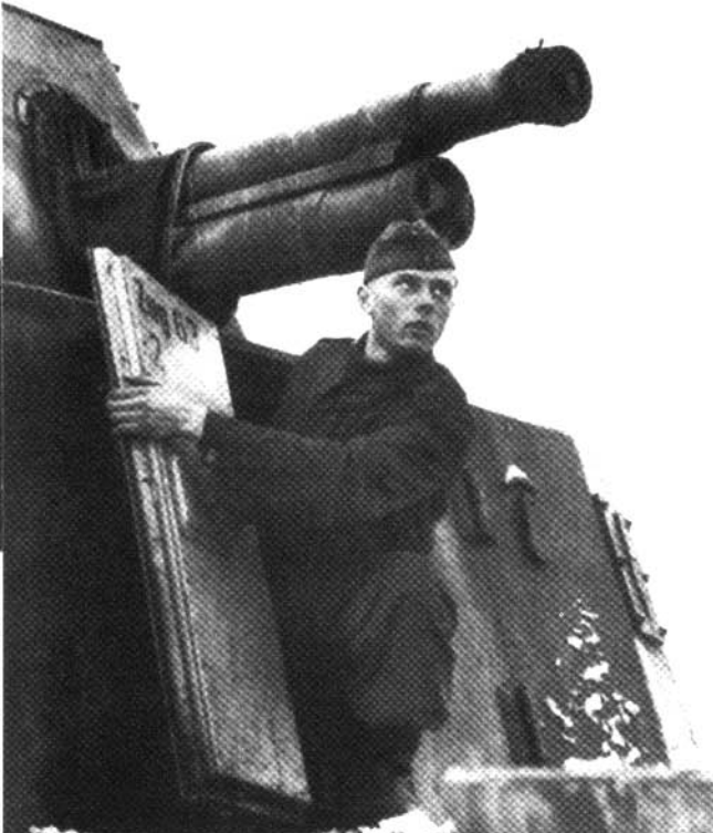
The guns of the BP 42 armored train. At left is the 7.62-cm 295/1(r) field cannon, the Russian M 02/30 with the shorter L/30 barrel (Vo 635 m/sec, maximum range 12 km); at right the Skoda 14/19 10-cm light field howitzer, from captured Polish and probably also from Czech material (Vo 395 m/sec, maximum range 9.8 km).(BA)
