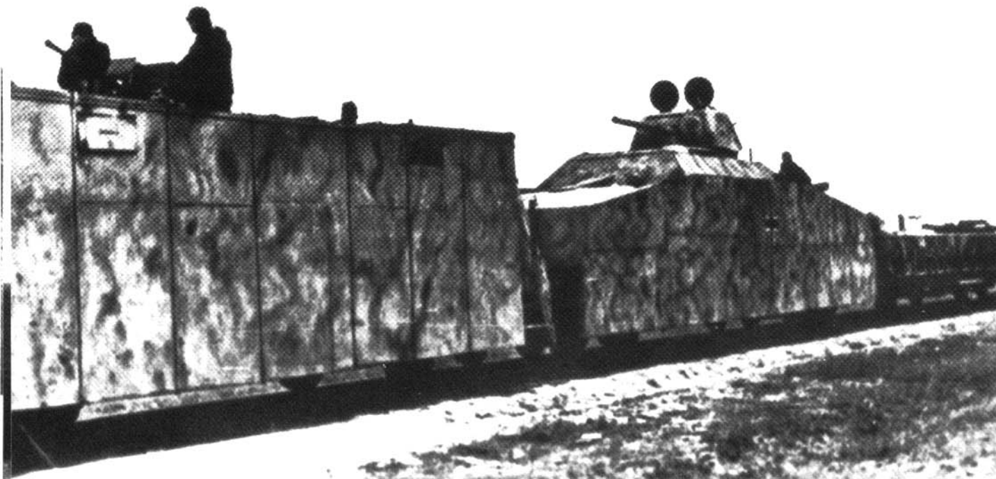
Above: The rail protection train formed in the early summer of 1942 by the 83rd Infantry Division bore the division's number as its own designation. It included two armored cars with the turrets of Russian BT-7 tanks (4.5-cm KwK) and remained in action until May of 1945.(HE)
